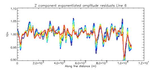
Figure 5: Tempest Line 6 Z component residuals. Early times in blue through to later times in red.
