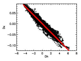
Figure 2. Scatterplot showing the dependence of the 385Hz amplitude residuals (Dx) on flying height residuals (Dh) before "height correction".
