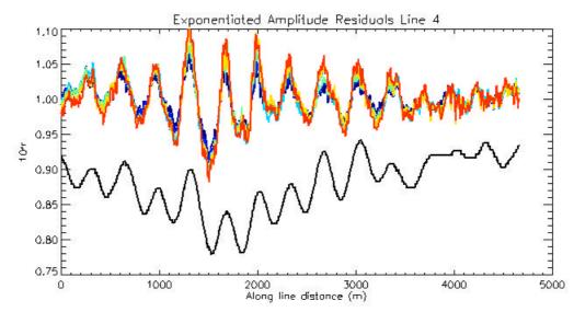
Figure 3. Dighem Line 4 amplitude residuals for all six frequencies. High frequency in red through to low in blue. The black profile is of the transverse correction, C, required to move the observation points onto the common line (rescaled, C/1000 + 0.9).
