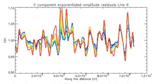
Figure 4: Tempest Line 6 X component residuals. Early times in blue through to later times in red.
